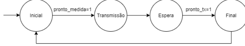
Figure 8: State transition diagram of the control unit.
