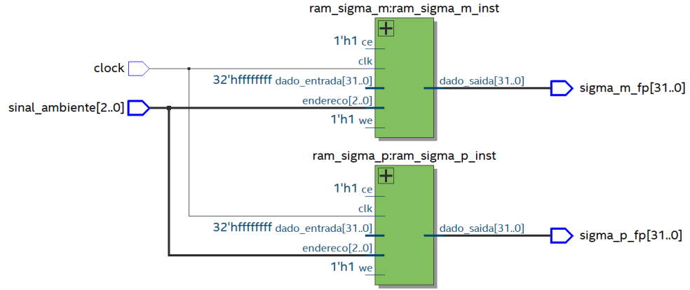
Figure 28: Block diagram of the environment decoding module - stores parameters \sigma_P and \sigma_M .
